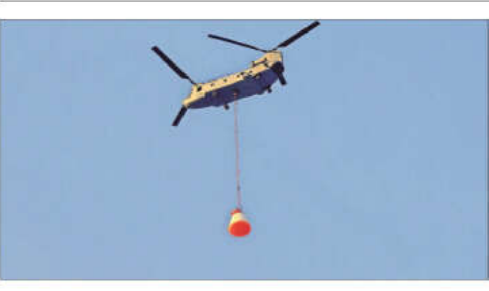
The air drop test with Gaganyaan-1 crew module was conducted off the Andhra Pradesh coast on Friday. CREDIT: ISRO
